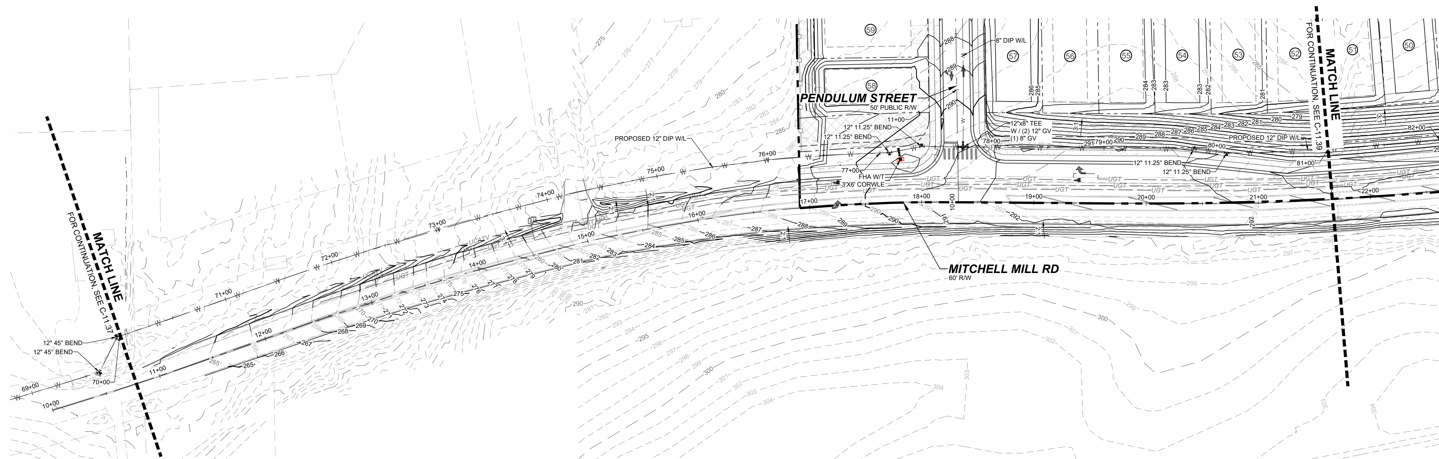
OFF-SITE WATER MAIN STATION 70+00 - 81+00 - PLAN HORIZONTAL: 1" = 50'
