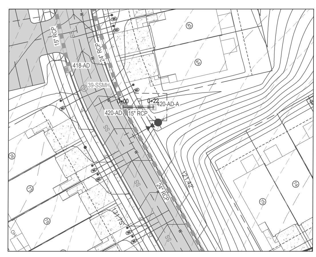
STORM SEWER - PLAN
