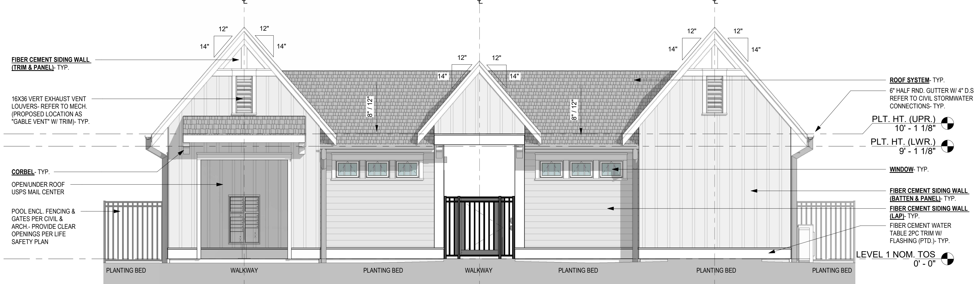
1 ELEVATION- POOLHOUSE FRONT (PARK SIDE) NEW A201 1/4" = 1'-0"
