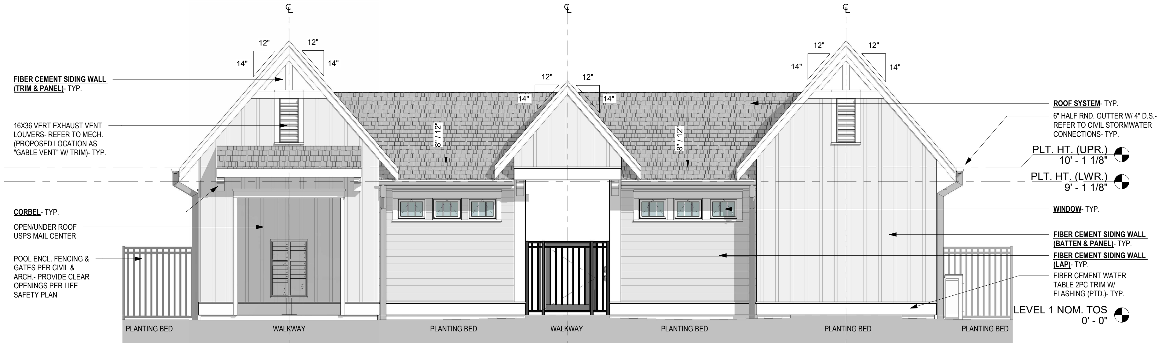
1 ELEVATION- POOLHOUSE FRONT (PARK SIDE) NEW A201 1/4" = 1'-0"
