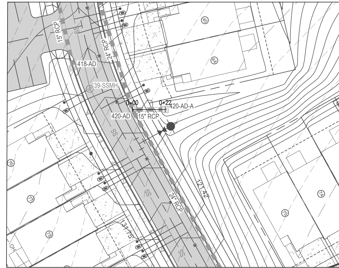
STORM SEWER - PLAN
