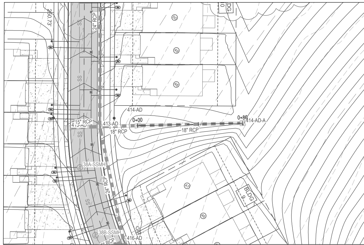
STORM SEWER - PLAN
