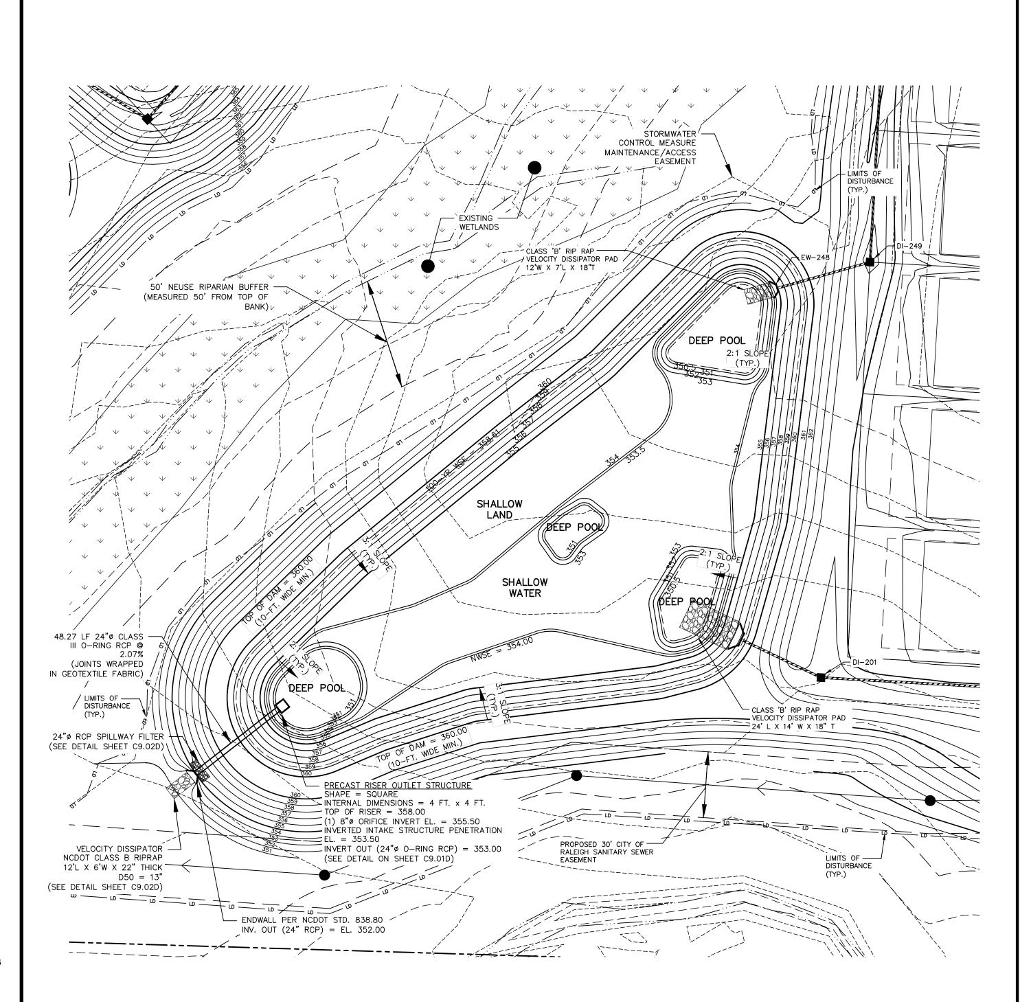
STORMWATER CONTROL MEASURE 'D' PLAN VIEW
